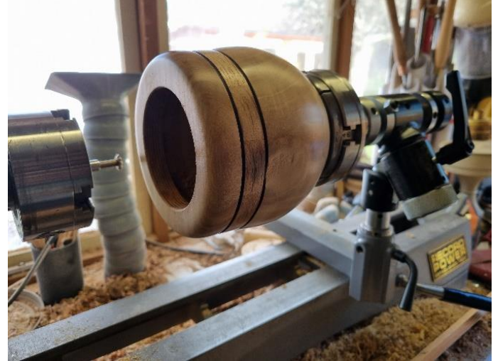
Fig. 3 - Jig pivoted back away from the cutter to allow checking of the thread
