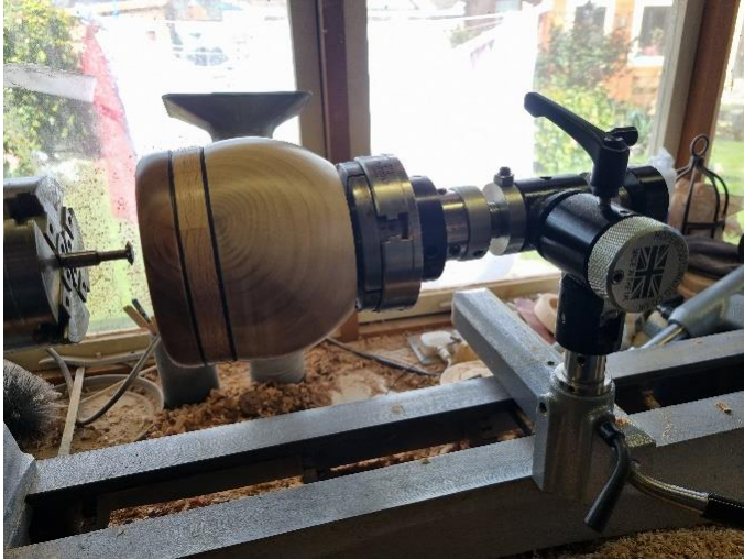
Fig. 2 - Jig carrying chuck and workpiece presented for cutting
