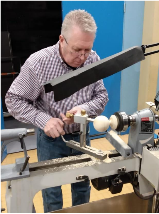
Vic Russell with his home-made sphere turning jig. He also showed how to finish off the sphere and had brought in his belt sander to compare with Alan's. (See article below for more detail)
