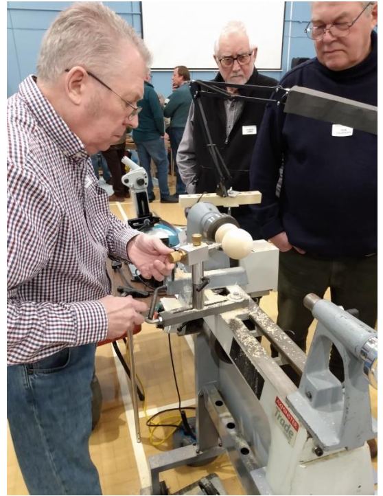
Vic Russell with his home-made sphere turning jig. He also showed how to finish off the sphere and had brought in his belt sander to compare with Alan's. (See article below for more detail)
