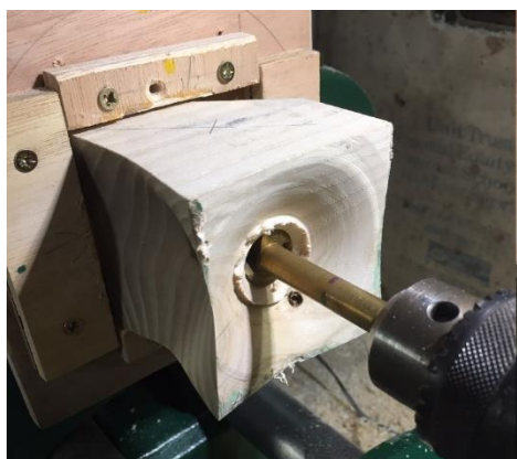
Drill to re-centre piece after it came loose
